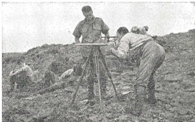
Making a "plane table" survey
